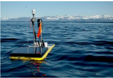
NOAA Carbon Wave Glider deployed in Alaska to help scientists better understand how melting glaciers affect the chemistry of the Prince William Sound. Credit: Wiley Evans
