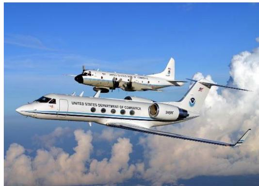
NOAA's Hurricane Hunters, the Gulfstream IV-SP jet (front) and Lockheed WP-3D Orion turboprop
